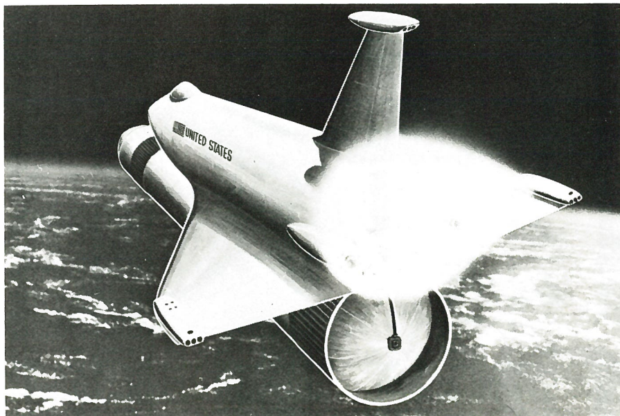
Figure 3. The selected space shuttle orbiter (see Fig. 1) with its external hydrogen/oxygen tank. The orbiter separates from its solid propellant boosters at 40 km altitude and continues on to an orbiting altitude of about 180 km, using its liquid propellant
