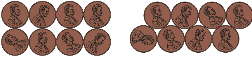
Figure 5. Three-dimensional foam problems can often be understood by considering their two-dimensional analogues. For a wet foam, the problem of minimizing the amount of foam material (or maximizing the amount of air) per unit volume reduces to a sphere-packing problem. The two-dimensional analogue of sphere-packing is circle-packing. At left, a square arrangement of disks (here, pennies) fills only 78.5 percent of the plane, whereas a hexagonal arrangement fills 90.7 percent. The hexagonal arrangement can be proved to be optimal.
