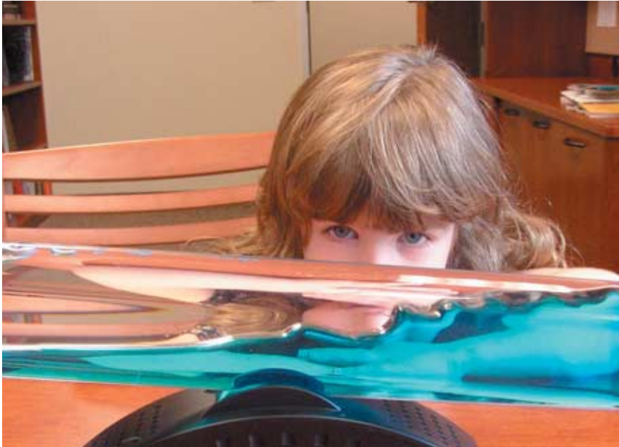
Figure 3. Novelty wave tank containing two liquids (one clear, one blue) of slightly different density demonstrates internal waves forming at the interface. Such waves appear to have strangely large amplitudes (compared with surface undulations of similar wavelength), and they seem to move slowly compared with water waves. Internal waves can also form even where no distinct interface exists: All that is needed is a vertical gradient in the density of the liquid.
