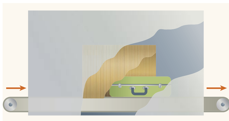
Figure 6. Current baggage scanners based on nuclear quadrupole resonance warn of the presence of hidden explosives; one day they may also show the approximate position of the suspect object (or objects) within a piece of luggage. The trick is to perform a series of measurements while a conveyor belt moves the suitcase into or out of the detection coil (above). Results for a test bag containing two explosive masses (as seen in the x-ray image, upper right) show the NQR signal diminishing in two steps as the bag moves out of the device (middle right). A simple algorithm that takes account of the physical parameters of the detection coil transforms these measurements into a form that shows the location of the hidden explosives within the bag (lower right).
