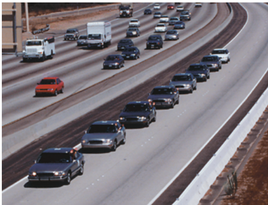
A "Look ma, no hands!" demonstration of automated driving took place in 1997 in San Diego, where eight Buick sedans cruised down Interstate 15 in close formation, with some of the "drivers" waving out the window to show they were not in control. The test cars are on a closed roadway (ordinarily used for high-occupancy-vehicle traffic); to help the cars stay in their lane, sensors on the underbody detect magnetic studs installed in the concrete. The demonstration was part of a program, sponsored by the U.S. Department of Transportation, that was canceled a year later. (Image courtesy of the National Automated Highway System Consortium.)
